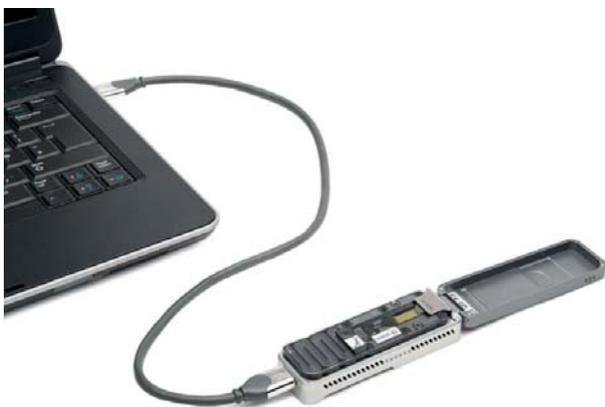
**Fig. 2.** ONT's MinION sequencing device attached to a laptop computer. With permission of Oxford Nanopore Techniques.
